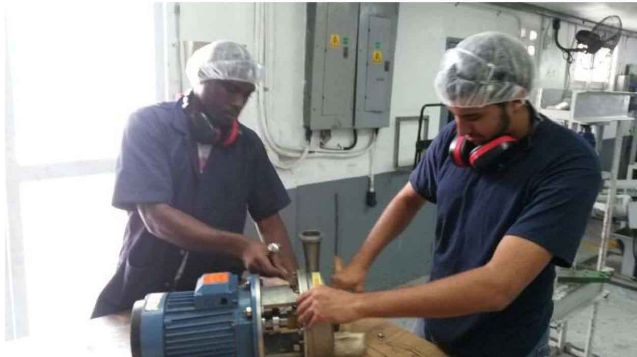
**CAP. 1(from left):** John St. Rose and Ramon Harper performing preventative maintenance to a Cleaning in Place (CIP) pump.
